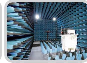
Full Anechoic EIRP Chamber
