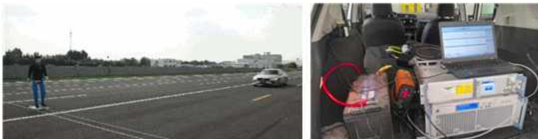
b) Outdoor BCI immunity test for the ADAS
