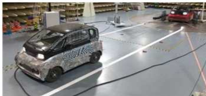
a) Indoor immunity test for the ADAS
