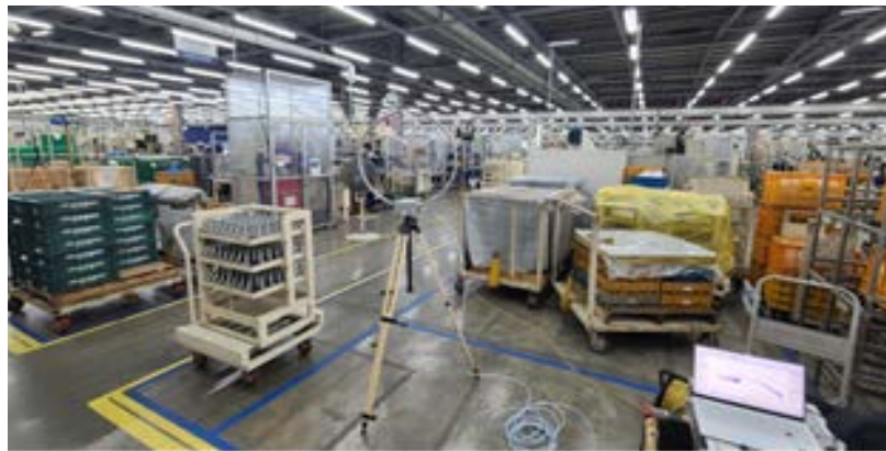
On-site measurement of EM wave intensity in the factories using Eum 5G
