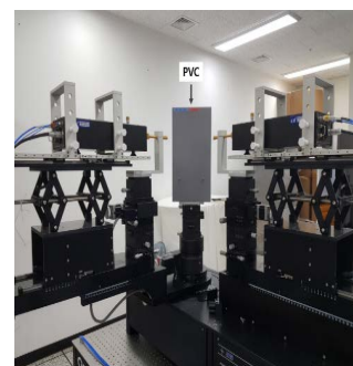
Terahertz-band radio propagation characteristics measurement system by material
