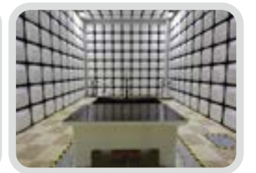
Electromagnetic anechoic chamber
